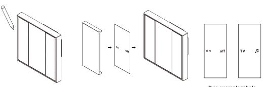
Step 1: Remove the white color central cover plate using a sharp tool such as tweezers.
